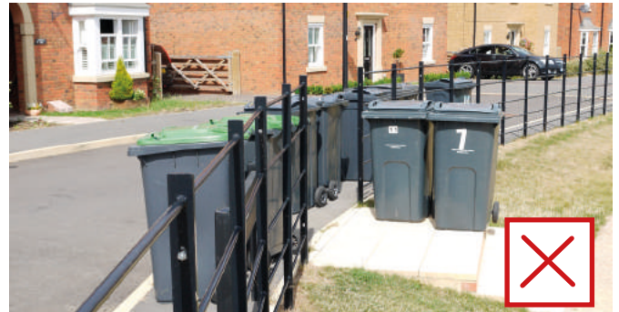
Footways / cycleways should not be expected to provide space for bin collection areas
